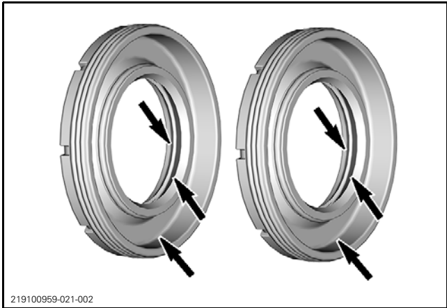
PUT GREASE IN ALL SEAL CAVITIES.
