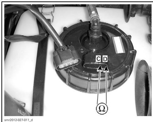
TYPICAL - FUEL LEVEL SENSOR RESISTANCE TEST
