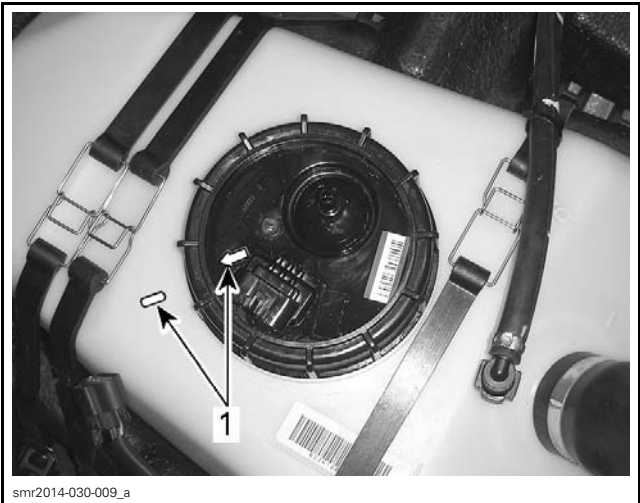
TYPICAL - FUEL PUMP MODULE INDEXING 1. Align marks
