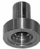
IMPELLER SHAFT PUSHER (P/N 529 035 955)
