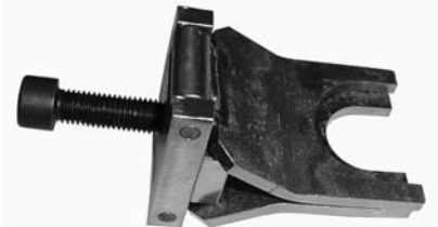
FLOATING RING TOOL (TYPE II) (P/N 529 036 116)
