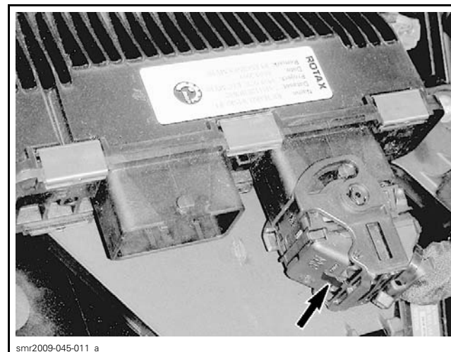
LOCKING TAB FULLY OUT
